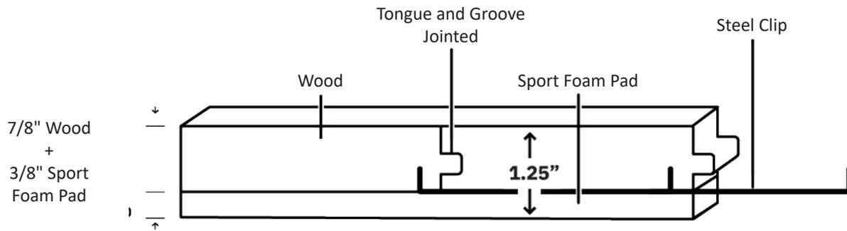
The 7/8" (22mm) solid hardwood floor boards are joined together with Steel Clips, which allow for unique independent floor board flexing. The floor floats over a 3/8" (10mm) performance foam underlay for maximum resilience
